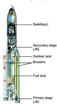
Bottom right: ESA's Ariane V rocket showing how fuel and oxidiser tanks make up the majority of a rocket. Credit: European Space Agency
