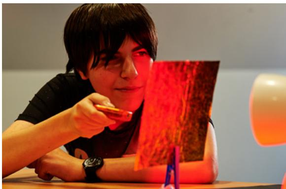
Participants investigate which material will do the best job of stopping heat from the Sun warming up the sensitive detectors on the Webb Telescope. In this demonstration, the IR lamp represents the Sun, and the IR thermometer represents the telescope.
